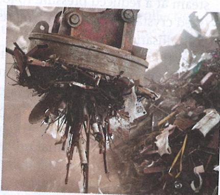
Figure 19 Separation using magnetism. The huge magnet on a crane at a refuse dump or demolition site lifts metal waste.
