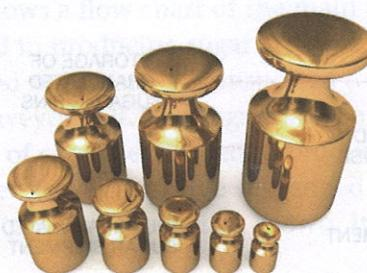
Figure 22 We can use a beam balance to measure the mass of anything that is within the range of weights to balance it. A balance compares mass with mass. So, a balance would give a correct measurement of mass on the moon, where the weights of the masses would be less than those on the earth.
