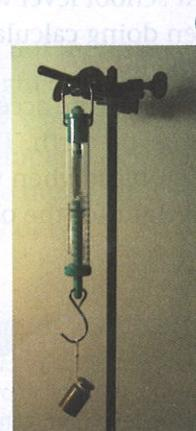
Figure 24 A: An example of a spring balance; B: A mass piece is weighed on a spring balance. A 1 kg mass piece has a weight of 10 newtons (N).
